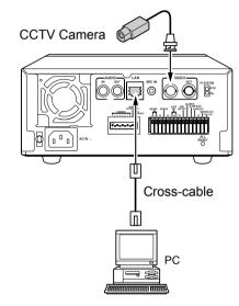
• To connect to an intranet (Use an Ethernet hub.)
